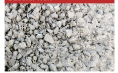
BUNDREX 65/35CH steel fibers are high quality structural steel fibers designed for reinforcement in shotcrete spraying. They are used successfully to replace the electro welded mesh in the reinforcement of tunnels, with an excellent performance proven with laboratory tests according to EN14651 and ASTM1609 standards.
