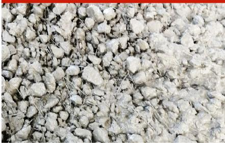
**BUNDREX 50/50 LH** steel fibers are high quality structural steel fibers designed for reinforcement in Slab On Grade. They are used successfully to replace the electro welded mesh in the reinforcement of industrial floors with an excellent performance proven with laboratory tests according to EN14651 and ASTM1609 standards.
