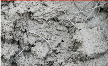
**SUPER BUNDREX 65/35 CA** steel fibers are high quality structural steel fibers designed for reinforcement in sprayed concrete. They are used successfully to replace the electro welded mesh in the reinforcement of tunnels, with an excellent performance proven with laboratory tests according to EN14651 and ASTM1609 standards.
