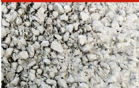
**BUNDREX 56/35CH** steel fibers are high quality structural steel fibers designed for reinforcement in shotcrete spraying. They are used successfully to replace the electro welded mesh in the reinforcement of tunnels, with an excellent performance proven with laboratory tests according to EN14651 and ASTM1609 standards.
